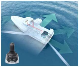
With the joystick the helmsmen can now maneuver the boat, in any direction at low speed with just one hand. The joystick is coupled to a sophisticated and specially developed software that individually commands the engines and the pod units to steer, throttle and shift gears independently, making the boat move in any direction the helmsmen wants – sideways, diagonally, forward, backward or rotate – with just one hand. Visit volvopenta.com to see for yourself!
