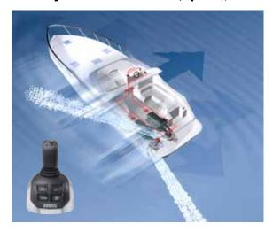
With the joystick the driver can maneuver the boat, at low speed. The joystick is coupled to a sophisticated and specially developed software that individually commands the electronically controlled engines and underwater units of the system to steer, throttle and shift gears independently, making the boat move in any direction the driver wants - sideways, diagonally, forward, backward or rotate - with just one hand. Visit volvopenta.com to see for yourself!
