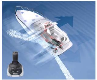
With the joystick the driver can now maneuver the vessel at low speed – with just one hand. The joystick is coupled to a sophisticated and specially developed software that individually commands the electronically controlled engines and underwater units of the system to steer, throttle and shift gears independently, making the boat move in any direction the driver wants – sideways, diagonally, forward, backward or rotate. Visit volvopenta.com to see for yourself!
