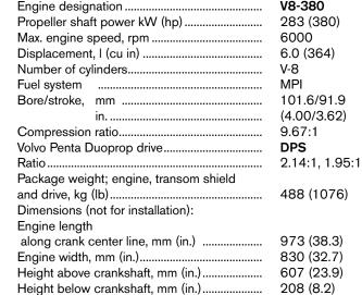
Propshaft power according to ISO 8665
